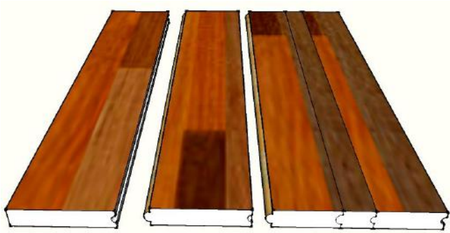
(a) (i) Tongue and Groove joint
